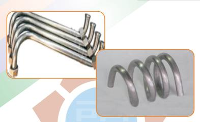
Bundy Tubing:- Bundy Tubes are Double Walled Copper Braised Tubes (DWCB) 0.7 mm thick, having great strength and ductility and also high resistance to vibration fatigue. It is ideally used for brake systems in automobiles, lubrication, pneumatics etc. Available in bends and fitting as per customer's requirement, with fitting of male & female nuts, banjo tee, with braised, ferrule of flared ends. Sizes:- 4.7, 6.8 & 10 mm
